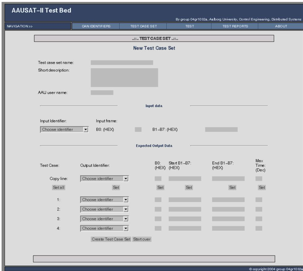
Figure 2.4: Screen-shot of the user interface for typing in a single frame test case set.
